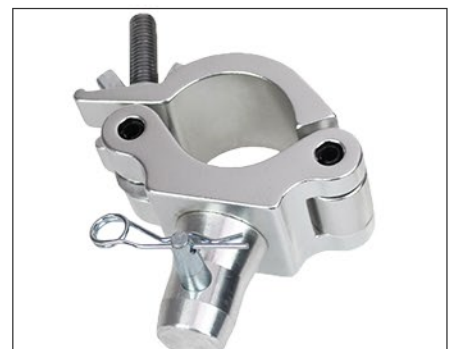
Halfcoupler connicle connect Diameter 48-51mm Width 50mm Loading 500kg
