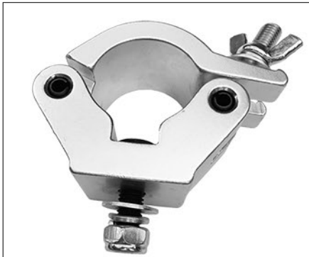
Heavy duty halfcoupler Diameter 48-51mm Width 50mm Loading 750kg
