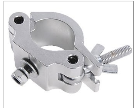
Halfcoupler Diameter 48-51mm Width 50mm Loading 500kg
