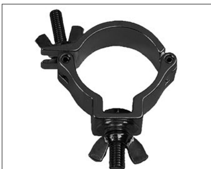
Light duty halfcoupler BL Diameter 48-51mm Width 30mm Loading 100kg
