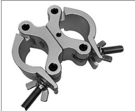
Swivel coupler Diameter 48-51mm Width 50mm Loading 500kg
