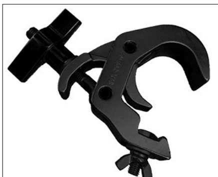
Quicktrigger BL Diameter 48-51mm Width 30mm Loading 250kg
