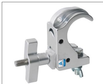
Quick clamp Diameter 50mm Width 30mm Loading 200kg
