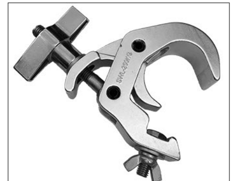
Quicktrigger Diameter 48-51mm Width 30mm Loading 250kg
