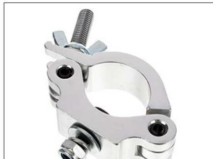
Halfcoupler small Diameter 48-51mm Width 30mm Loading 200kg
