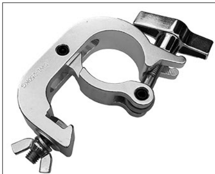
Trigger clamp Diameter 48-51mm Width 30mm Loading 300kg
