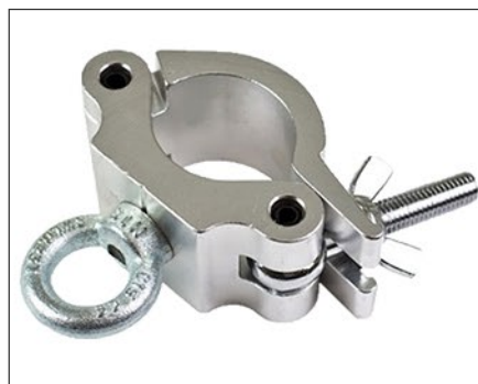
Halfcoupler lifting eye Diameter 48-51mm Width 50mm Loading 200kg
