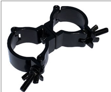
Swivel coupler light duty BL Diameter 48-51mm Width 30mm Loading 100kg
