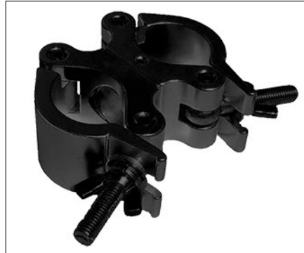
Swivel coupler BL Diameter 48-51mm Width 50mm Loading 500kg
